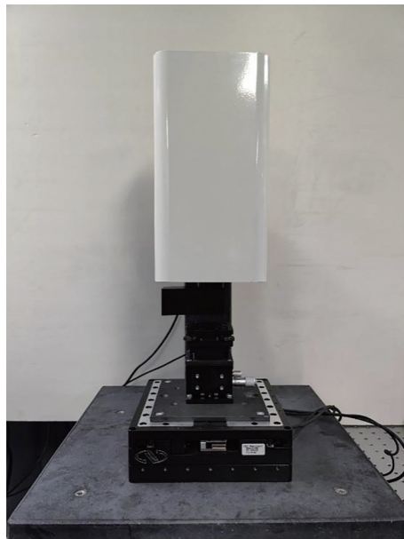
图6 大视场白光干涉测量系统装置 Fig. 6 Apparatus of large field-of-view white light interferometer
