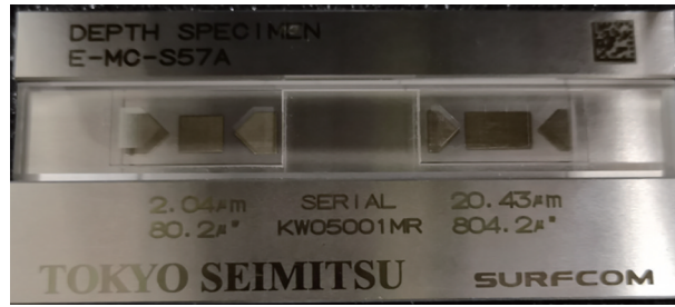
图9 标准台阶实物照片 Fig. 9 Photo of the standard step sample
